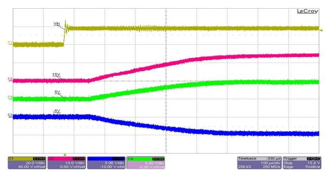
Test condition: The input voltage was set at 24V, and all outputs were set at full load. Ch1 - Vin, Ch2 – 15VP (+15V), Ch3 – 5VN (-5V), Ch4 – 5VP (5V)
