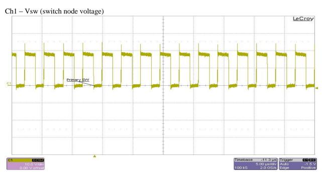
Test condition: The input voltage was set at 24V, and all outputs were set at full load.
