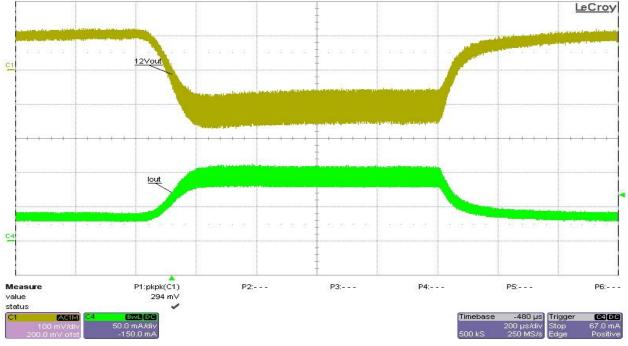
Test condition: Vin = 24V, 24VP (+24V) load from 0A to 25mA, no load at the other outputs. Ch1- 24VP (+24V) (AC mode), Ch4- Io (+24V output current)
