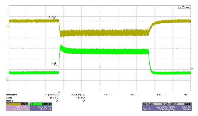
Test condition: Vin = 24V, 12VN (-12V) load from 0A to 50mA, no load at the other outputs. Ch1- 12VP (-12V) (AC mode), Ch4- Io (-12V output current)
