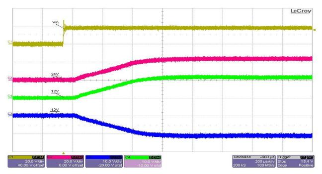
Test condition: The input voltage was set at 24V, and all outputs were set at full load. Ch1 - Vin, Ch2 - 24VP (+24V), Ch3 - 12VN (-12V), Ch4 - 12VP (+12V)
