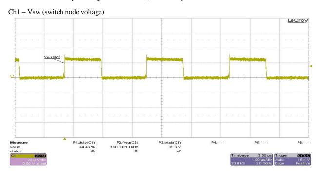
Test condition: The input voltage was set at 30V, and all outputs were set at full load.
