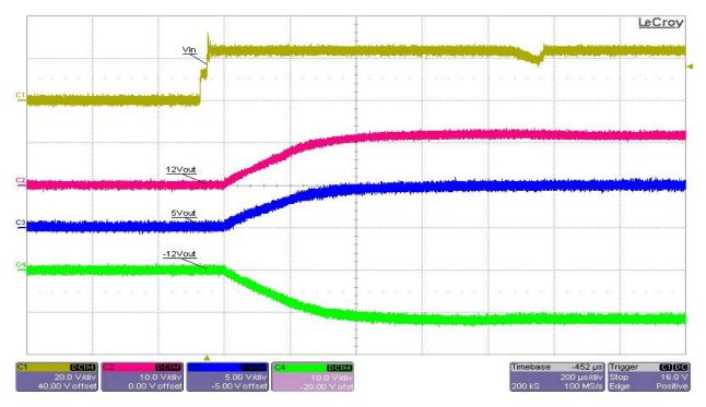
Test condition: The input voltage was set at 30V, and all outputs were set at full load. Ch1 - Vin, Ch2 – 12VP (+12V), Ch3 – 5VP (+5V), Ch4 – 12VN (-12V)
