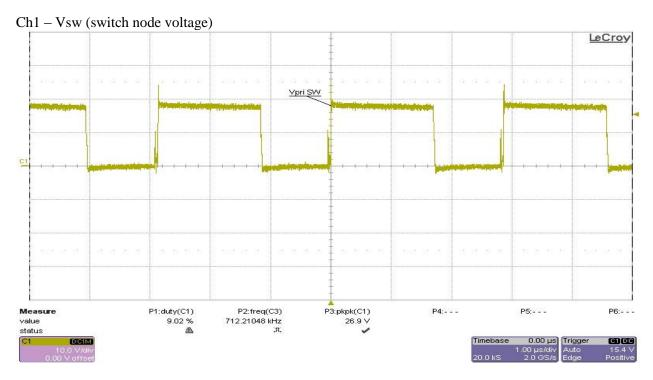
Test condition: The input voltage was set at 24V, and all outputs were set at full load.
