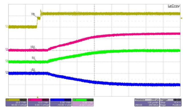
Test condition: The input voltage was set at 30V, and all outputs were set at full load. Ch1 - Vin, Ch2 – 15VP (+15V), Ch3 – 5VN (-5V), Ch4 – 5VP (5V)
