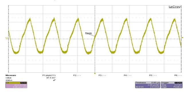
Test condition: The input voltage was set at 24V, and all outputs were set at full load. Ch1 - 12VP (+12V) (AC coupled)
