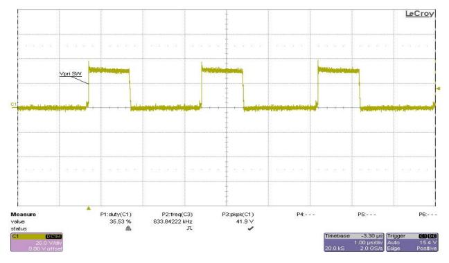
Test condition: The input voltage was set at 30V, and all outputs were set at full load.
