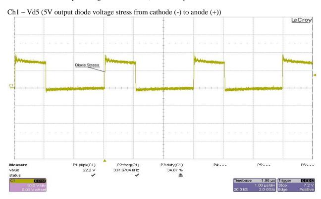
Test condition: The input voltage was set at 30V, and all outputs were set at full load.
