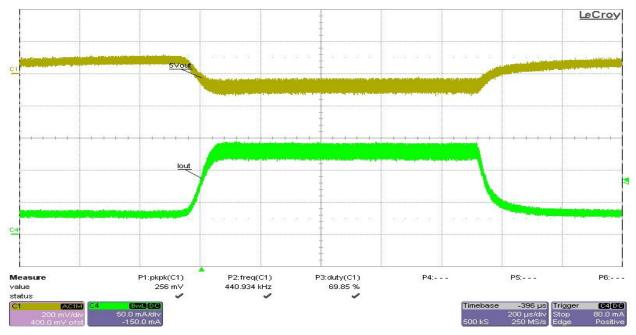
Test condition: Vin = 24V, 15VP (+15V) load from 0A to 50mA, no load at the other outputs. Ch1- 15VP (+15V) (AC mode), Ch4- Io (+15V output current)
