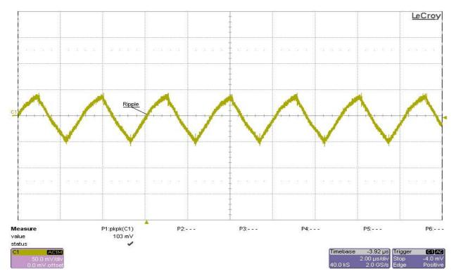
Test condition: The input voltage was set at 24V, and all outputs were set at full load. Ch1-12VN (-12V) (AC coupled)
