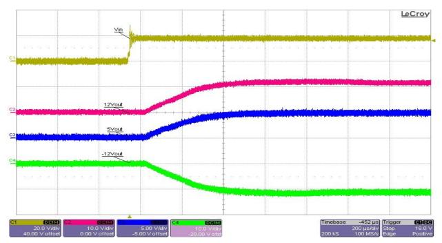
Test condition: The input voltage was set at 24V, and all outputs were set at full load. Ch1 - Vin, Ch2 – 12VP (+12V), Ch3 – 5VP (+5V), Ch4 – 12VN (-12V)
