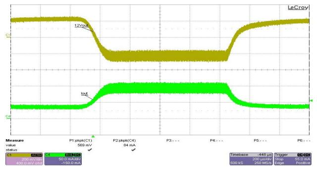
Test condition: Vin = 24V, 5VP (+5V) load from 0A to 100mA, no load at the other outputs. Ch1- 5VP (+5V) (AC mode), Ch4- Io (+5V output current)
