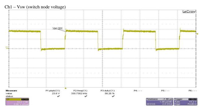
Test condition: The input voltage was set at 24V, and all outputs were set at full load.
