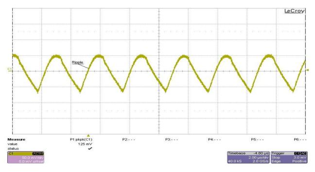
Test condition: The input voltage was set at 24V, and all outputs were set at full load. Ch1-5VN (-5V) (AC coupled)
