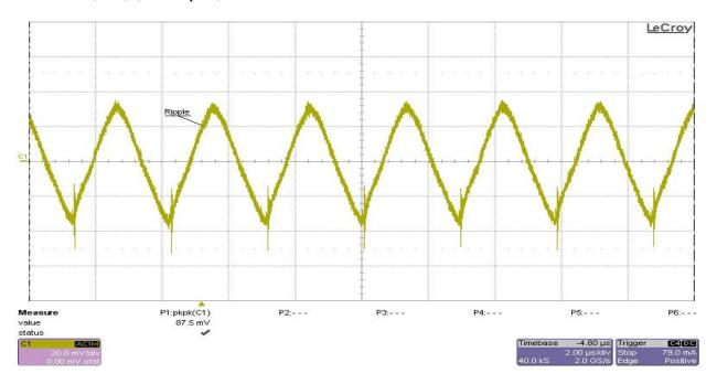
Test condition: The input voltage was set at 24V, and all outputs were set at full load.  $Ch1-15VP\ (+15V)\ (AC\ coupled)$
