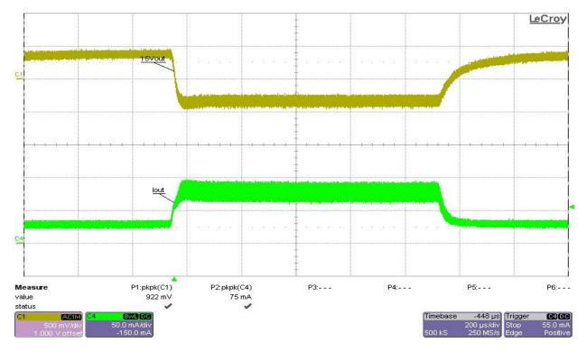
Test condition: Vin = 24V, 5VN (-5V) load from 0A to 100mA, no load at the other outputs. Ch1- 5VN (-5V) (AC mode), Ch4- Io (-5V output current)
