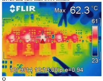
Thermal Image: 12.0163Vin 0.9977Vout 326kHz/phase 14.735ain 160.046aout 90.2% 5" fan 12.0V 460mA at 5" from UUT 30 minutes stabilized 23 deg. C ambient IR729 and 50 max U301 hottest
