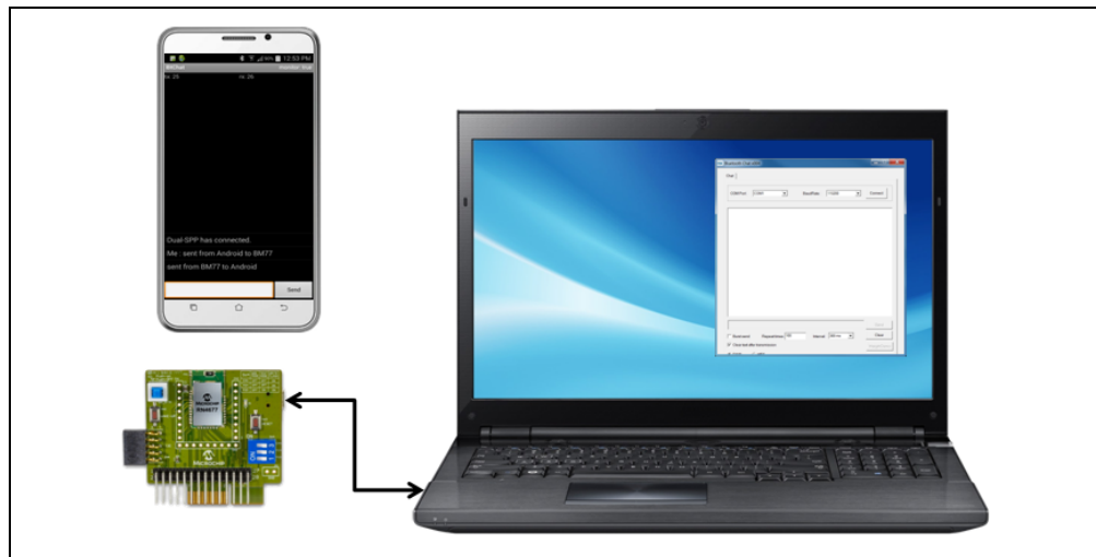
FIGURE 2-1: BLUETOOTH® SPP CONNECTION TO SMARTPHONE
