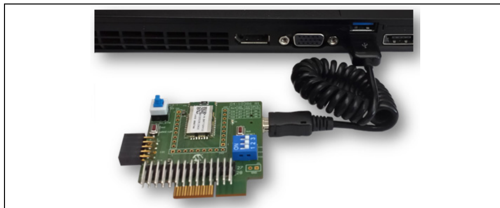
FIGURE 2-2: CONNECT THE BM77 PICtail™ BOARD TO A HOST PC USB PORT
