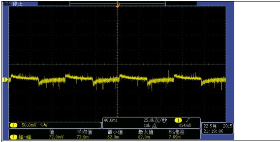
Vin:198Vac test condition: 50%-100% of full load, 0.1A/us, 100ms cycle
