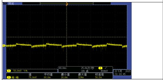
Vin:242Vac test condition: 50%-100% of full load, 0.1A/us, 100ms cycle
