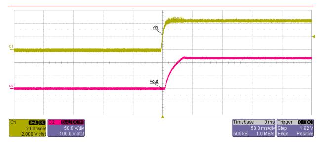
Startup into No Load at 5 Vin
