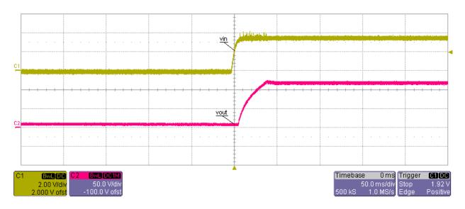
Startup into No Load at 3.5 Vin
