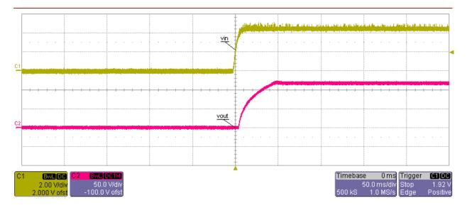
Startup into Full Load(10mA) at 5 Vin
