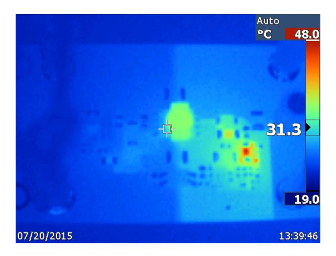
IR thermal image taken at steady state with 3.5 Vin and 120V@10mA output
