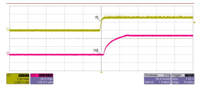
Startup into Full Load(10mA) at 3.5 Vin
