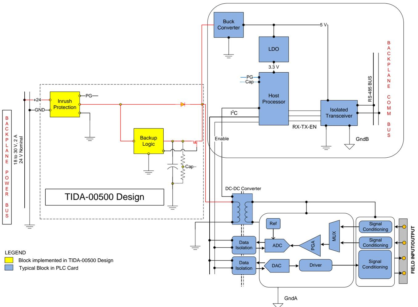
Figure 1. Generic Illustration of Power Block
