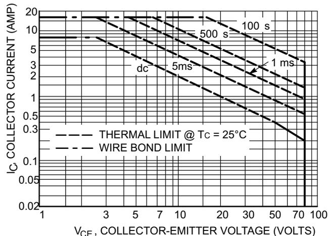
**Figure 6. SOA of Transistor**
