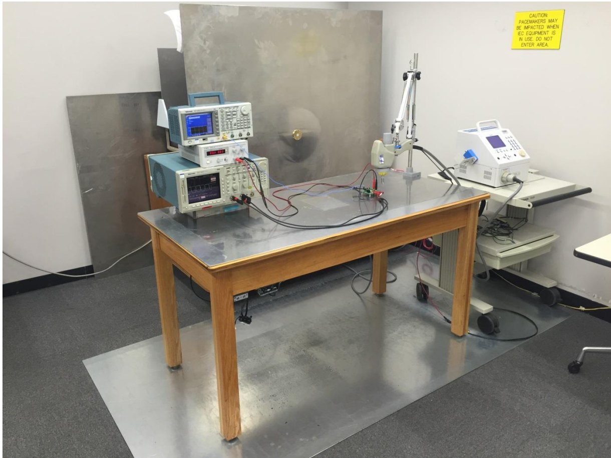
Figure 6: IEC ESD Compliant Test Setup
