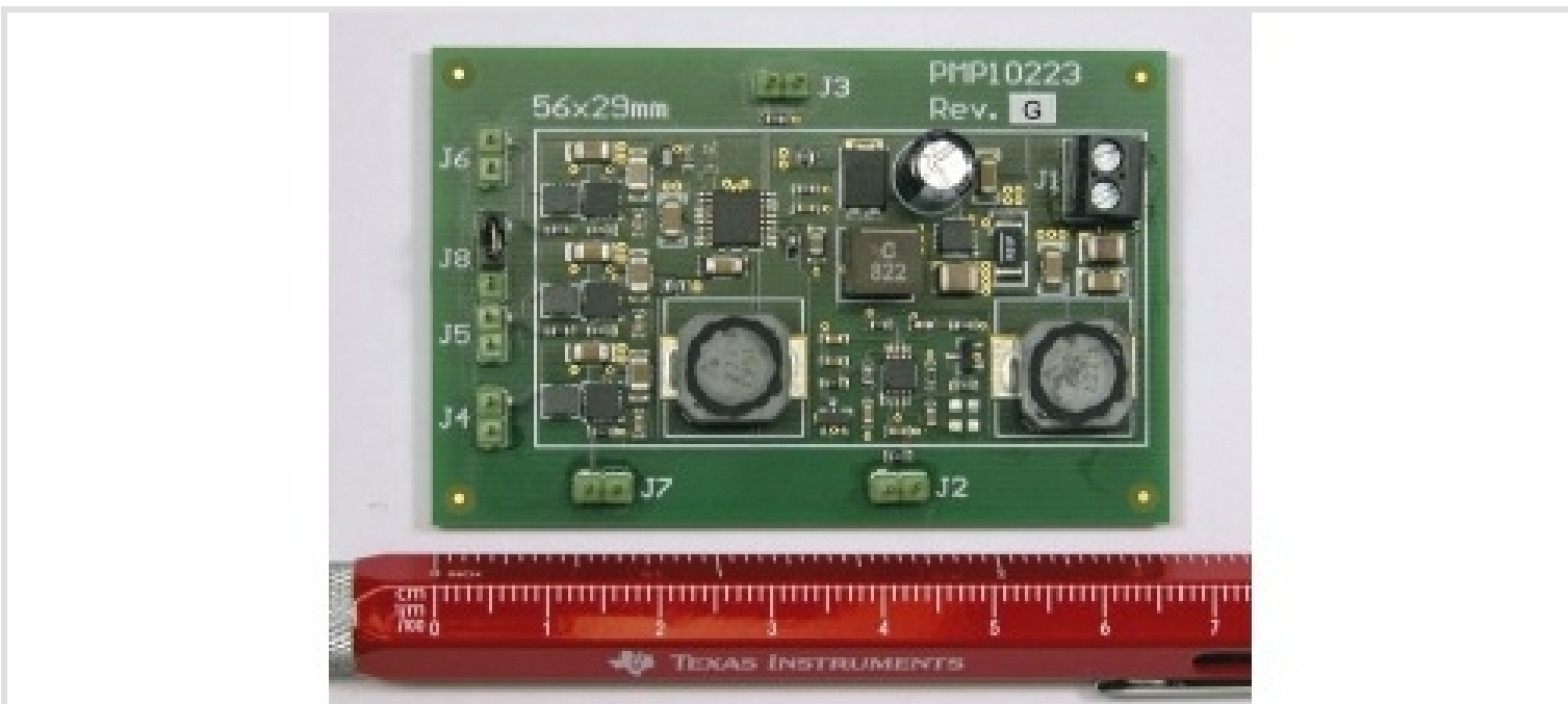
PMP10223.1 Automotive Power Supply with Pre-Boost Reference Design Board Image
