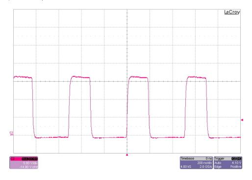
The photo below shows the FET switching voltage (TP3) for an input voltage of 7.25V and a 2A load. (5V/DIV, 200nS/DIV)
