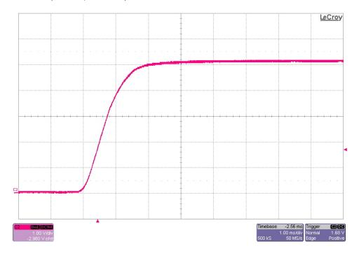
The photo below shows the output voltage startup waveform after the application of 12V in. The 5V output was loaded to 2A. (1V/DIV, 1mS/DIV)
