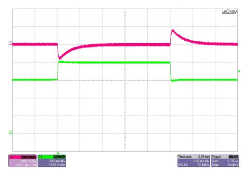
The photo below shows the 5V output voltage (ac coupled) when the load current is stepped between 1A and 2A. Vin = 12V. (200mV/DIV, 500mA/DIV, 1mS/DIV)
