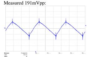
Input ripple across J1, 48Vin 50mV/div; 2usec/div
