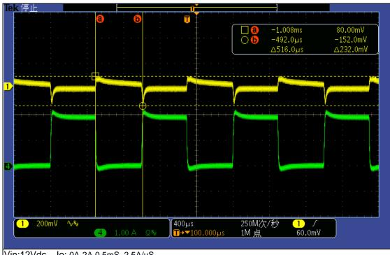
Vin:12Vdc lo: 0A-2A 0.5mS, 2.5A/uS Ch1: Output Ripple Voltage 200mV/div
