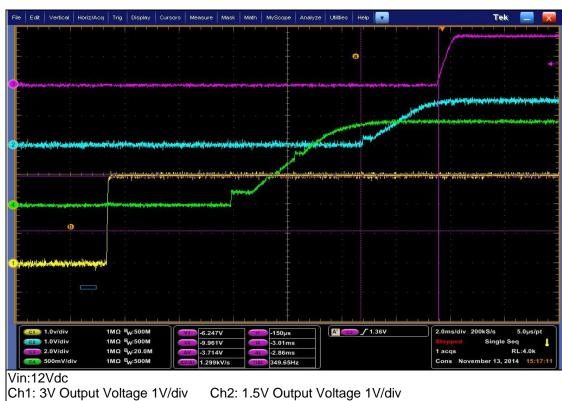
Ch3: 3.3V Output Voltage 2V/div Ch4: 1.425V Output Voltage 500mV/div
