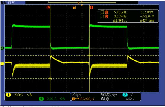
Vin:12Vdc Io: 0A-4A 0.5mS, 2.5A/uS Ch1: Output Ripple Voltage 200mV/div
