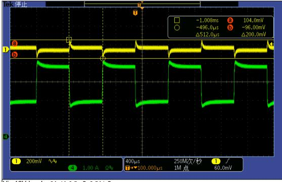
Vin:12Vdc Io: 2A-4A 0.5mS, 2.5A/uS Ch1: Output Ripple Voltage 200mV/div
