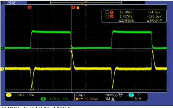
Vin:12Vdc Io: 0A-1.5A 0.5mS, 2.5A/uS Ch1: Output Ripple Voltage 100mV/div
