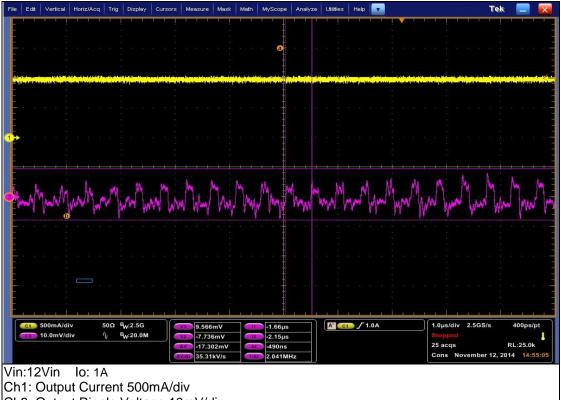
Ch3: Output Ripple Voltage 10mV/div
