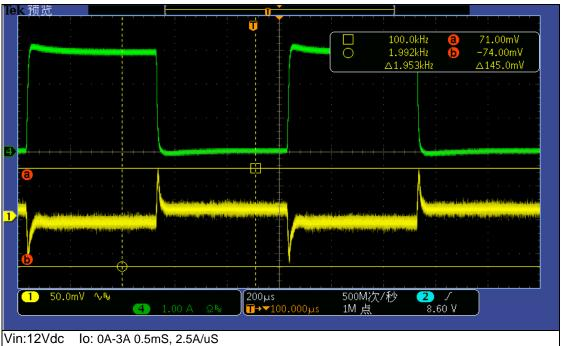
Vin:12Vdc Io: 0A-3A 0.5mS, 2.5A/uS Ch1: Output Ripple Voltage 50mV/div
