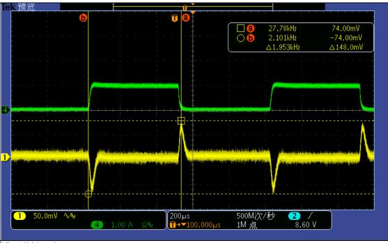
Vin:12Vdc Io: 0A-1A 0.5mS, 2.5A/uS Ch1: Output Ripple Voltage 50mV/div
