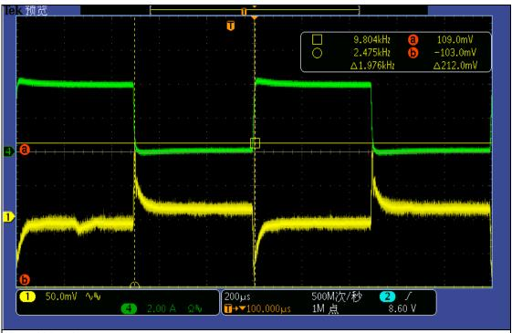
Vin:12Vdc lo: 0A-4A 0.5mS, 2.5A/uS Ch1: Output Ripple Voltage 50mV/div
