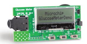
The analog front end—which incorporates an op amp, a precision ADC and a very accurate voltage reference—is embedded in the PIC16LF1786. Inbuilt DAC is used to properly bias the sensor. A Real-Time Clock/Calendar (RTCC) is used to record the time stamp, and the internal EEPROM stores up to 32 readings for later reference via the LCD. The XLP feature on this family of devices addresses the low power requirements.
