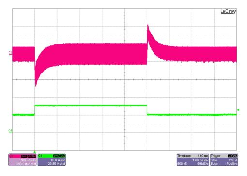
The photo below shows the 18V output voltage (ac coupled) when the load current is stepped between 5A and 15A. Vin = 12V. (500mV/DIV, 10A/DIV, 1mS/DIV)
