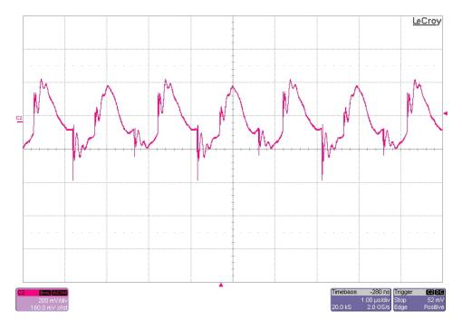
The 18V output ripple voltage (AC coupled) is shown in the figure below. The image was taken with the output loaded to 15A. The input voltage is set to 12V. (100 mV/DIV, 1 uS/DIV)
