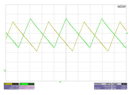
The photo below shows the measured inductor current in each phase. The input voltage was set to 12V with a 0A load. (2A/DIV, 1uS/DIV)
