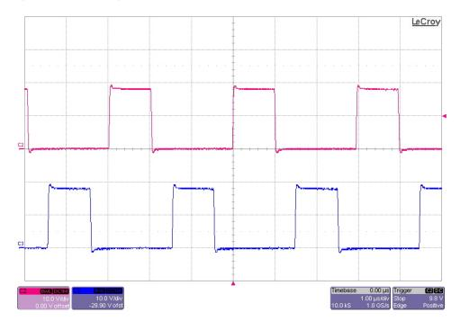
The photo below shows the FET switching voltages (TP2 top, TP9 bottom) for an input voltage of 15V and a 0A load. (10V/DIV, 1uS/DIV)
