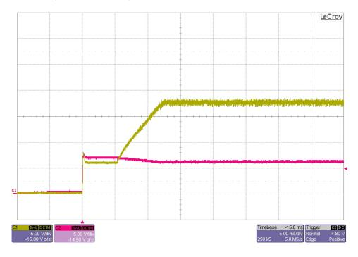
The photo below shows the output voltage startup waveform after the application of 15V in. The 18V output was loaded to 15A. (5V/DIV, 5mS/DIV)
