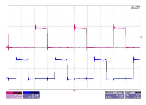
The photo below shows the FET switching voltages (TP2 top, TP9 bottom) for an input voltage of 15V and a 15A load. (10V/DIV, 1uS/DIV)
