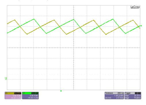
The photo below shows the measured inductor current in each phase. The input voltage was set to 12V with a 15A load. (5A/DIV, 1uS/DIV)
