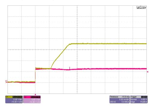
The photo below shows the output voltage startup waveform after the application of 15V in. The 18V output was loaded to 0A. (5V/DIV, 5mS/DIV)
