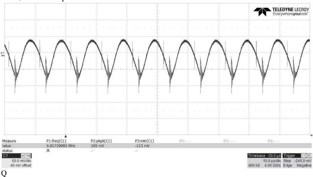
Ripple out at 1.5A load measured at main output J2 terminals: Vin is 32V Vout is 4.985V 106mV p-p ripple, slightly less at lower Vin's
