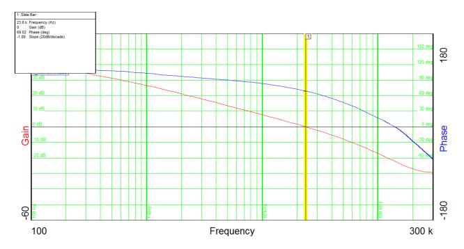
Output power = 3.3 V@0.42 AInput voltage = 8.0 VDCPhase margin  $= 69^{\circ}$ Bandwidth = 23.8 kHz
