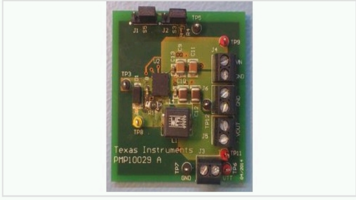
Reference Design - DDR3/DDR4 Power Supply with 5V Input and 10A Load for Industrial PCs
