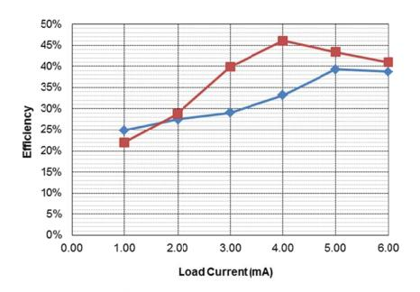
120VAC/60Hz -240VAC/60Hz 120VAC/60Hz lin Pout Losses Vin Pin (mW) PF Efficiency lout (mA) Vout (mArms) (mW) (mW) 0.000 4.53 119.9 0.15 0.00 0.0% 9 9 1.00 3.73 119.9 0.20 15 0.56 3.73 11 24.9% 3.71 0.35 27 0.62 7.42 20 27.5% 2.00 119.9 119.9 27 29.1% 3.00 3.68 0.47 38 0.68 11.04 4.00 3.65 119.9 0.52 44 0.71 14.60 29 33.2% 5.00 119.9 0.54 46 0.73 18.05 39.2% 3.61 28 6.00 3.61 119.9 0.62 56 0.72 21.66 34 38.7% 240VAC/60Hz lin Pout Losses
