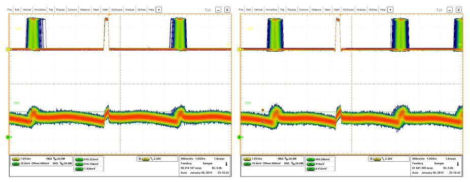
Load 0A Ripple: 8mV Load 20A Ripple: 8.5mV
