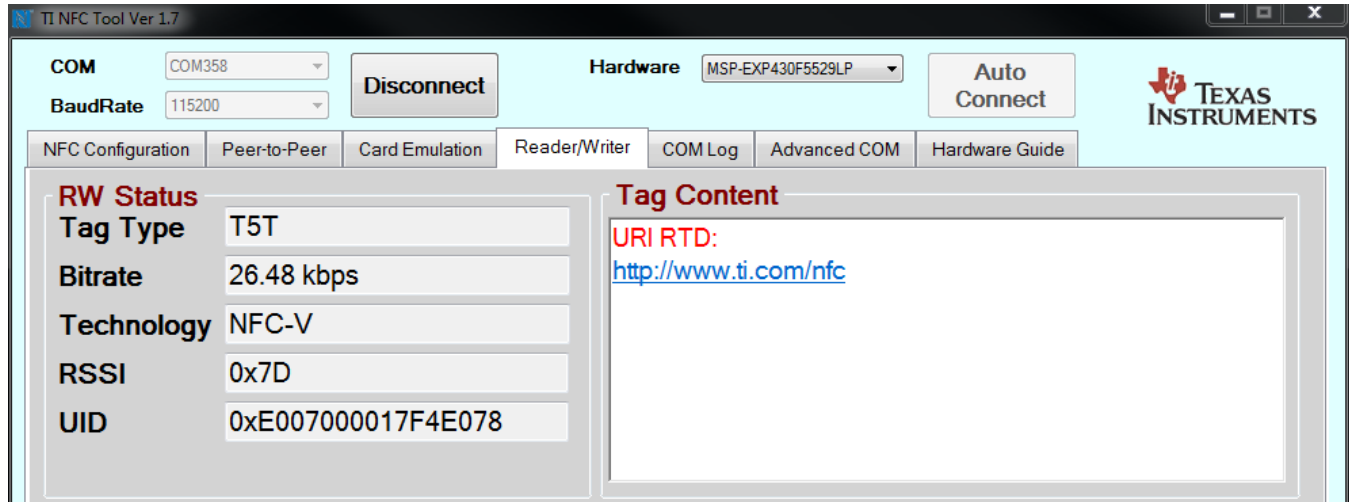
Figure 25. Reading NDEF Content of NFC Type 5 Tag Platform (URI RTD)
