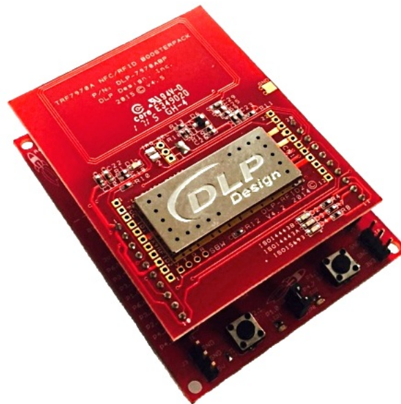
Figure 11. MSP-EXP430F5529LP + DLP-7970ABP Configuration
