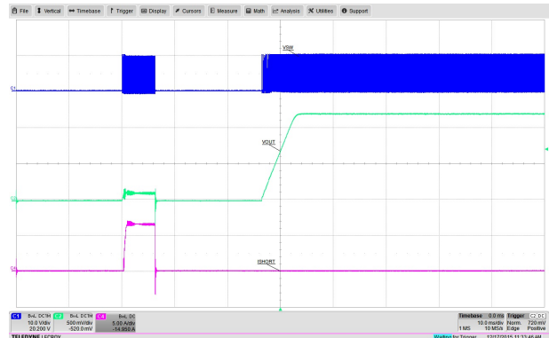
10Vin, 1.2Vout1, Short circuit released
