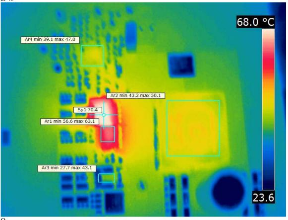
Snubber R (10 ohms) was size 2010. Based upon minimal heating, it can be size 1210 or even size 1206.
