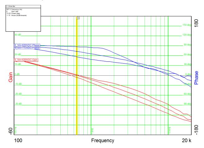
Input voltage = 325VDC: Phase margin =  $73^{\circ}$ Bandwidth = 0.657kHz
