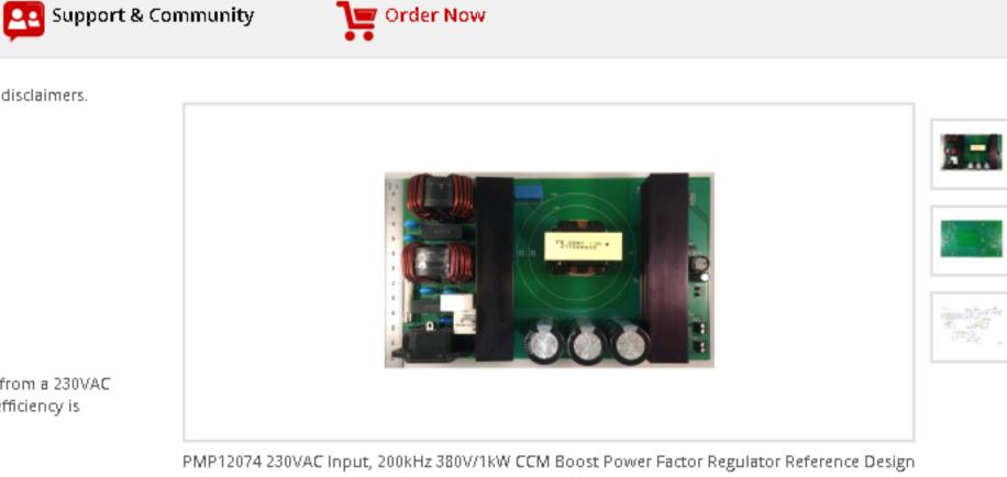
PMP12074 230VAC Input, 200kHz 380V/1kW CCM Boost Power Factor Regulator Reference Design Top of Board Image
