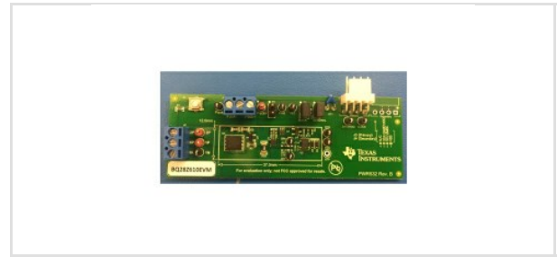
TIDA-00895 1 to 2s I2C Li-Ion Battery Pack Manager Reference Design Board Image
