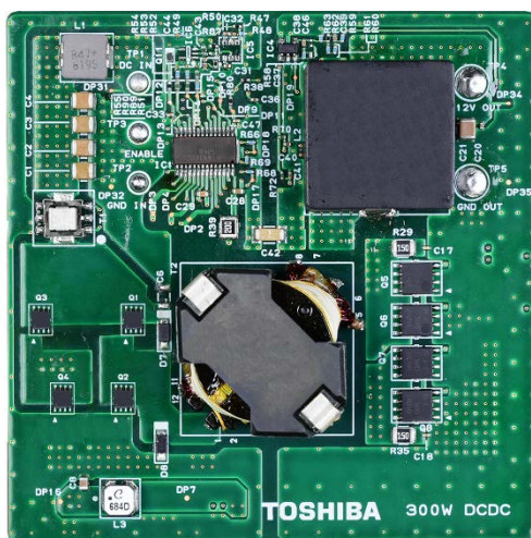
Figure 2.1 300W isolated DC-DC converter
