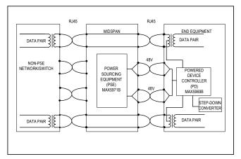
Figure 3. PoE midspan power injector.
