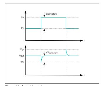
Figure 12. Output load step response.
