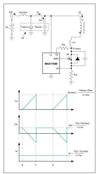
Figure 10. Primary-side circuit and currents.
