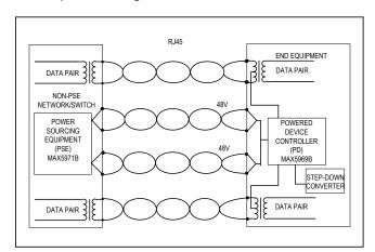
Figure 2. PoE endspan power injector.
