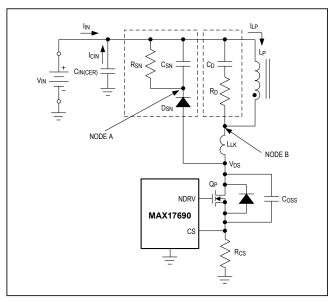
Figure 8. RCD snubber circuit.
