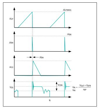
Figure 9. RCD snubber circuit waveforms.
