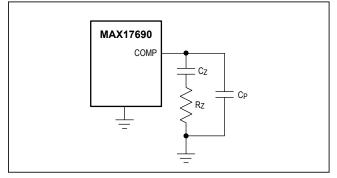
Figure 14. Type II compensation for OTA.
