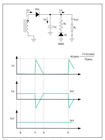
Figure 11. Secondary-side circuit and currents.
