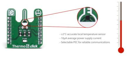
One shot reading allows for the lowest power consumption - down to 5uA, if there is no demand for continuous temperature conversion. The device remains in standby state, as long as there is no read command. Read command (writing 1 to the bit 0 of the config register) will wake up the device
