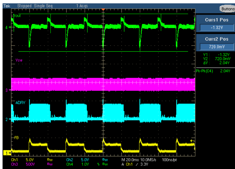
Figure 38 115 VAC 20 Vout Transient
