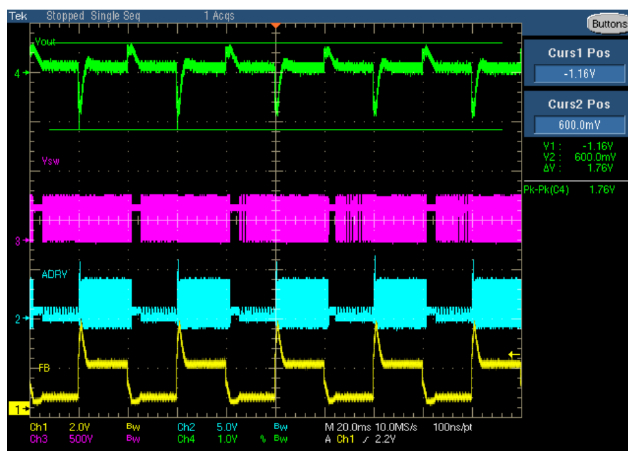
Figure 37 230 VAC 15 Vout Transient
