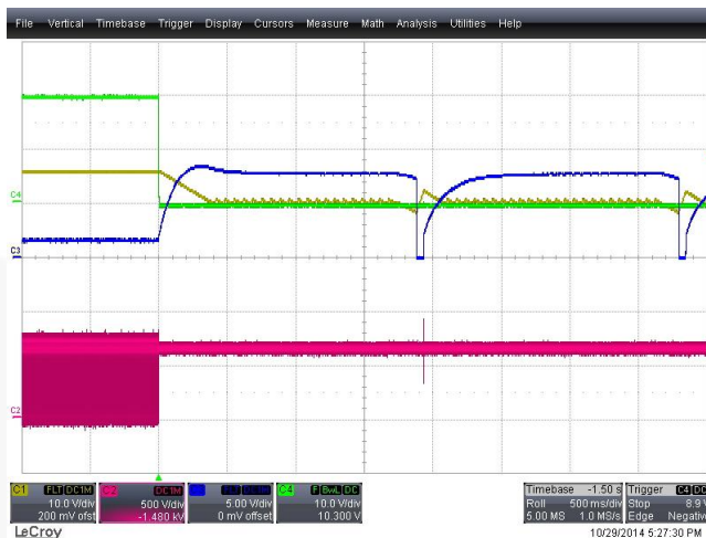
Figure 47. AOCB Triggered, Output Short with 460 V AC , Full-Load, (CH1: V CC (10 V/div), CH2: V DS (500 V/div), CH3: V FB (5 V/div), CH4: V OUT (10 V/div), Time: 500 ms/div)
