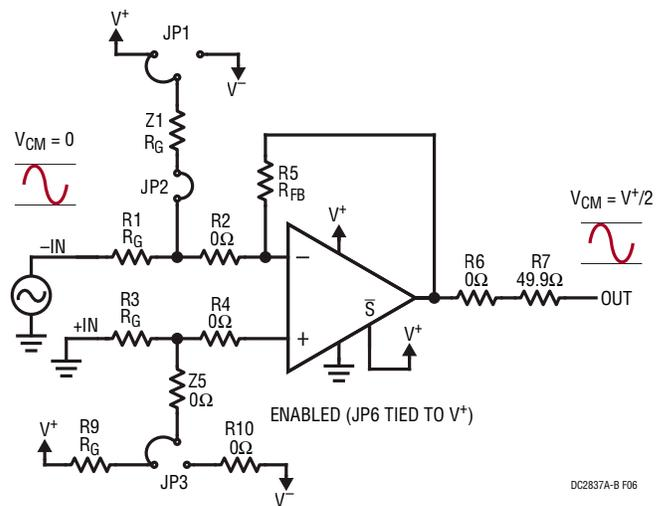
**Figure 6. Inverting Gain with DC Bias**
