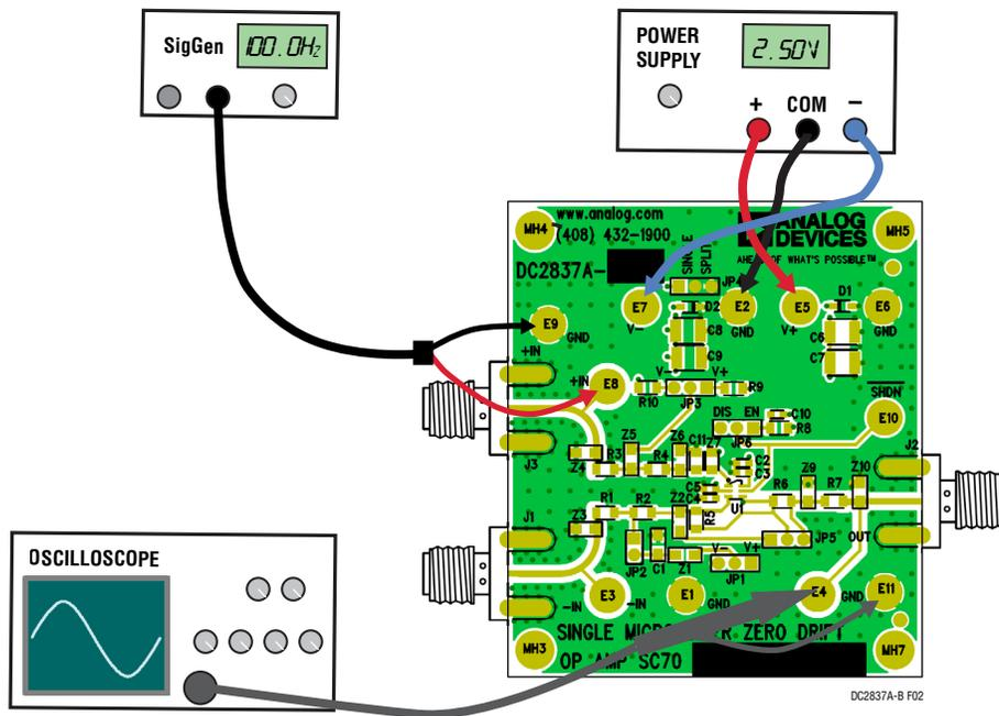
Figure 2. Proper Measurement Equipment Setup
