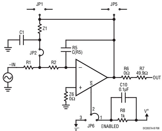
**Figure 8. Building A Second-Order Active Lowpass Filter with DC2837A**
