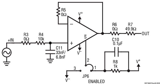
Figure 3. Unity Gain with +IN Lowpass Filter
