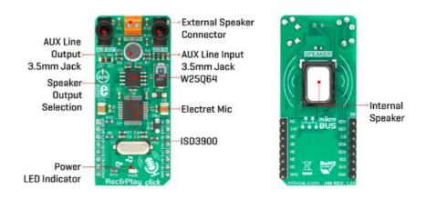
To allow the out-of-box functionality, the Click board  $^{\intercal}$  is equipped with a small omnidirectional electret microphone, along with a miniature  $8\Omega$  speaker.
