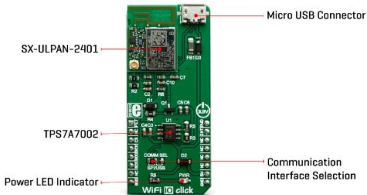
The ULPAN-SB-2401 module supports IPv4, TCP, and UDP transfer protocols, and complies with the IEEE802.11a/b/g/n wireless networking standards, at 2.4GHz. It supports data rates from 1 to 54 Mbps for 802.11b/g, and MCS from 0 to 7, for 802.11n. The SX-ULPAN-2401 module also provides support for WPS, WPA, and WPA2 security protocols, allowing a secure connection.
