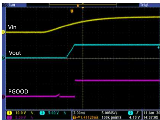
Figure 22. Power Up and PGOOD, No Load
