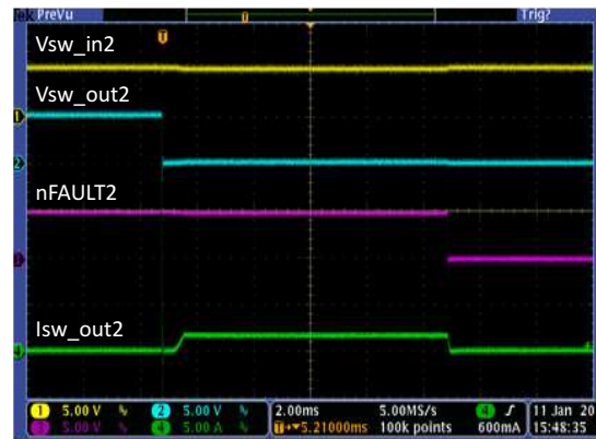
Figure 31. Power Switch2 Current Limit Operation
