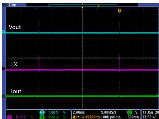
Figure 20. Buck Hiccup Response to Hard-Short Circuit
