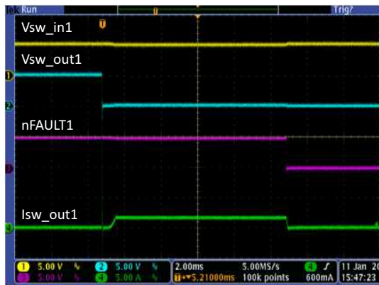
Figure 30. Power Switch1 Current Limit Operation
