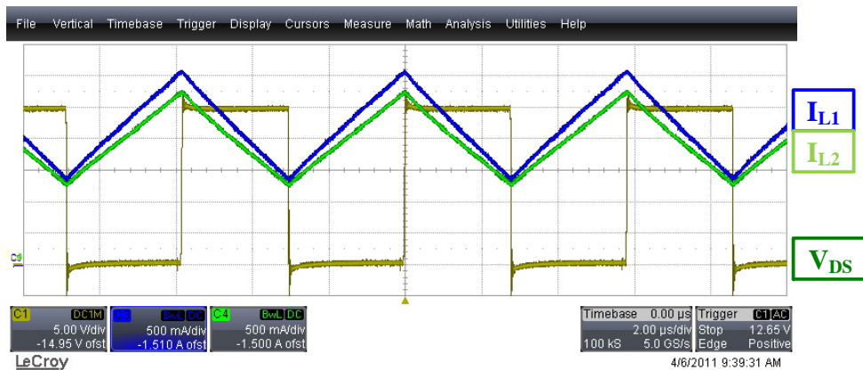
Figure 4. Operational Waveforms, V_{IN} = 12\text{ V} , R_{OUT} = 6\ \Omega
